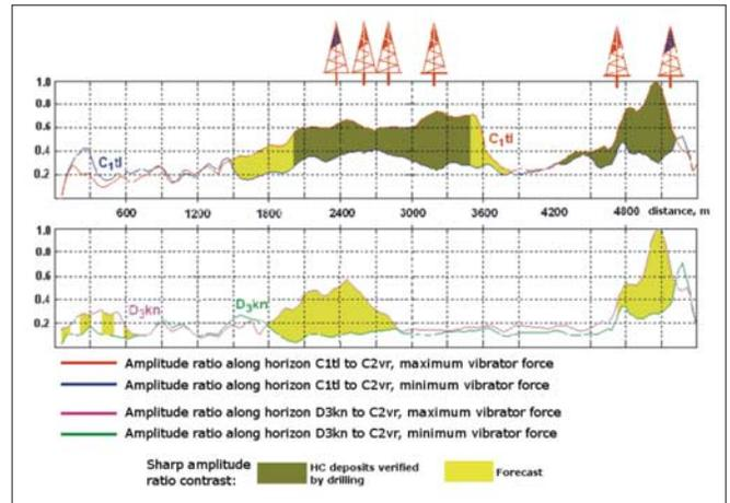
Figure 3. Variation in amplitude ratio of reflected waves for C1tl and D3kn to the amplitude of C2vr horizon with different forces at the source.
