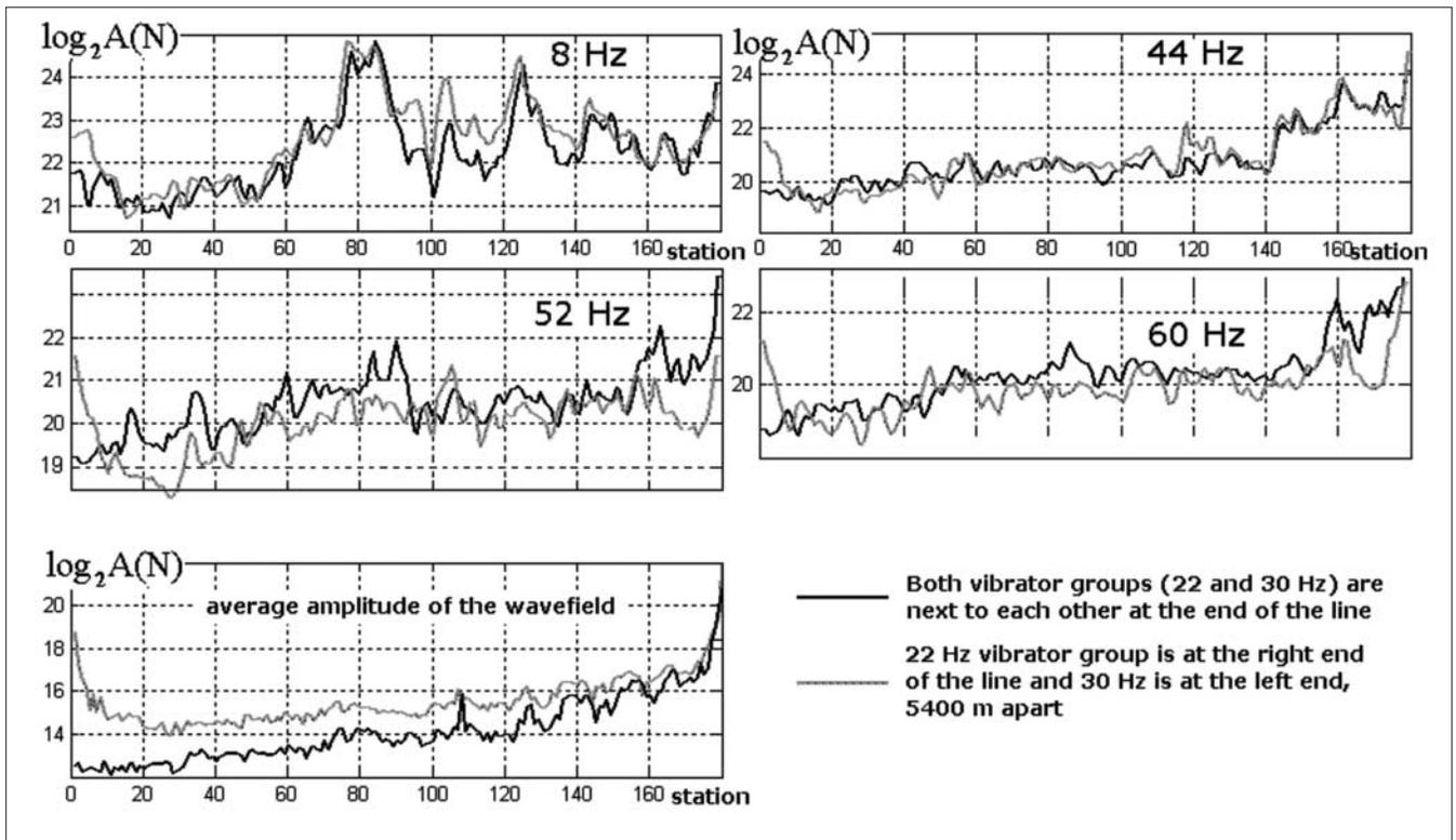
Figure 9. Amplitude variation of the nonlinear wavefield component based on the vibrator group location.
