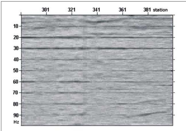
Figure 1. Example of a spectrogram for a wavefield acquired with two monochromatic signals: 20 and 30 Hz.
