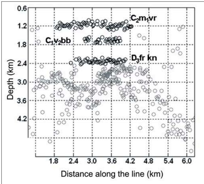
Figure 5. Distribution of seismic emission sources in the lower half-space for frequencies 2.8–6.4 Hz.
