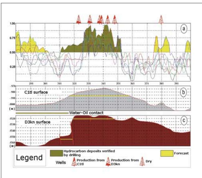
Figure 2. Amplitudes of a nonlinear component of the wavefield (a) with hydrocarbon-bearing horizons C1tl (b), and D3kn (c).
