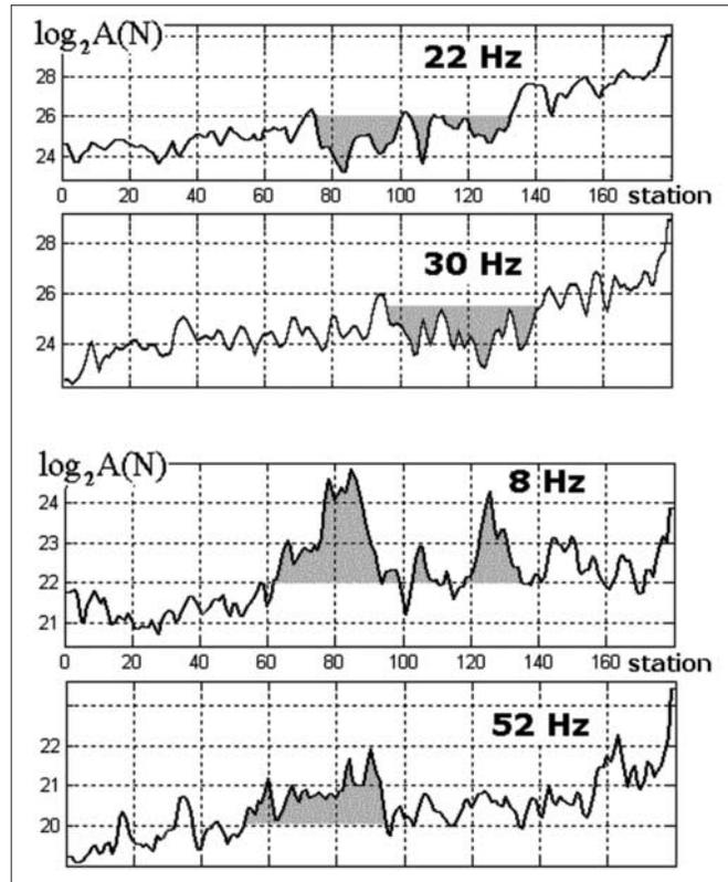
Figure 7. Amplitude variation for base and combinational frequencies. Both groups of vibrators are close to each other and at the end of the line.
