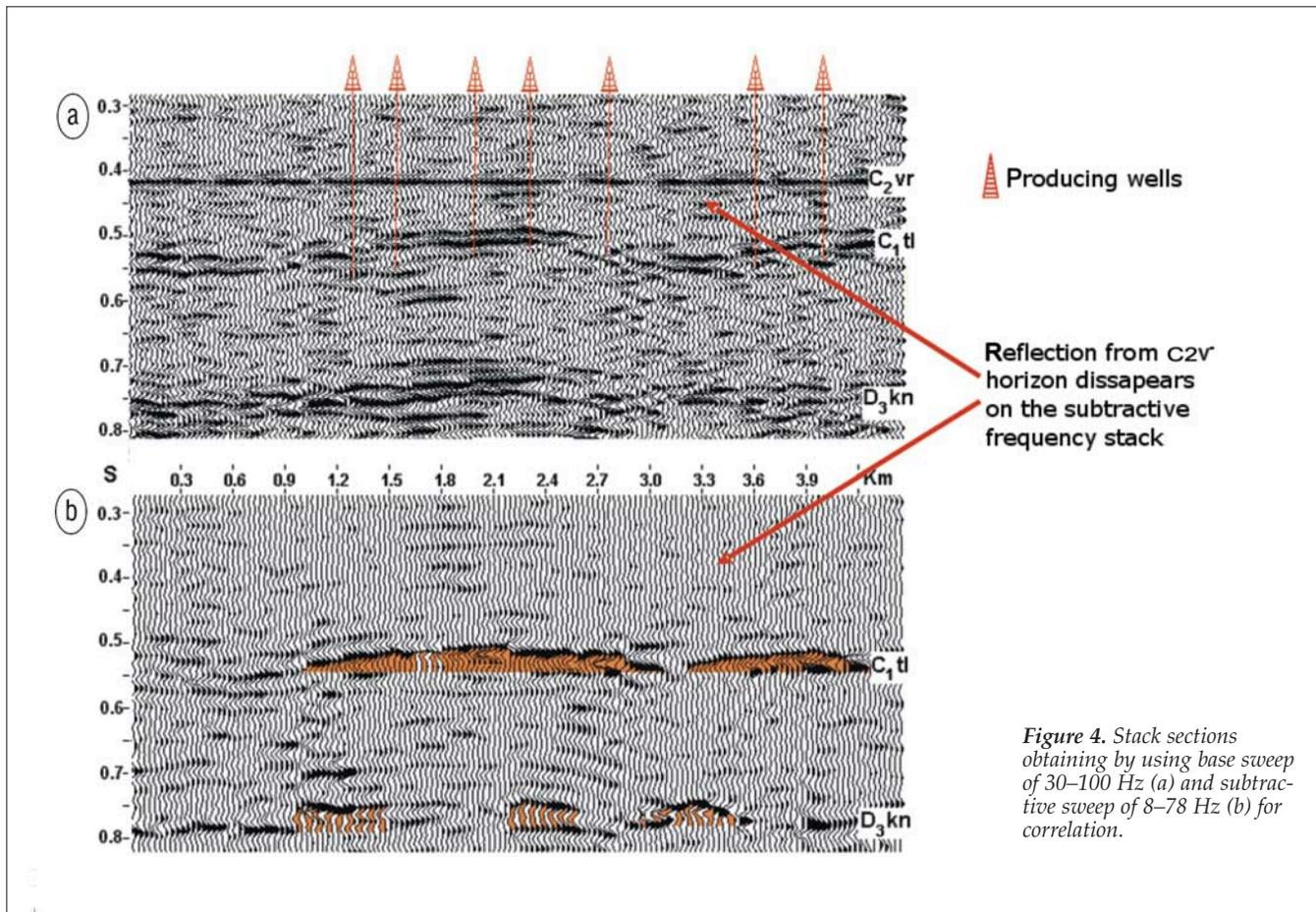
Figure 4. Stack sections obtaining by using base sweep of 30–100 Hz (a) and subtractive sweep of 8–78 Hz (b) for correlation.
