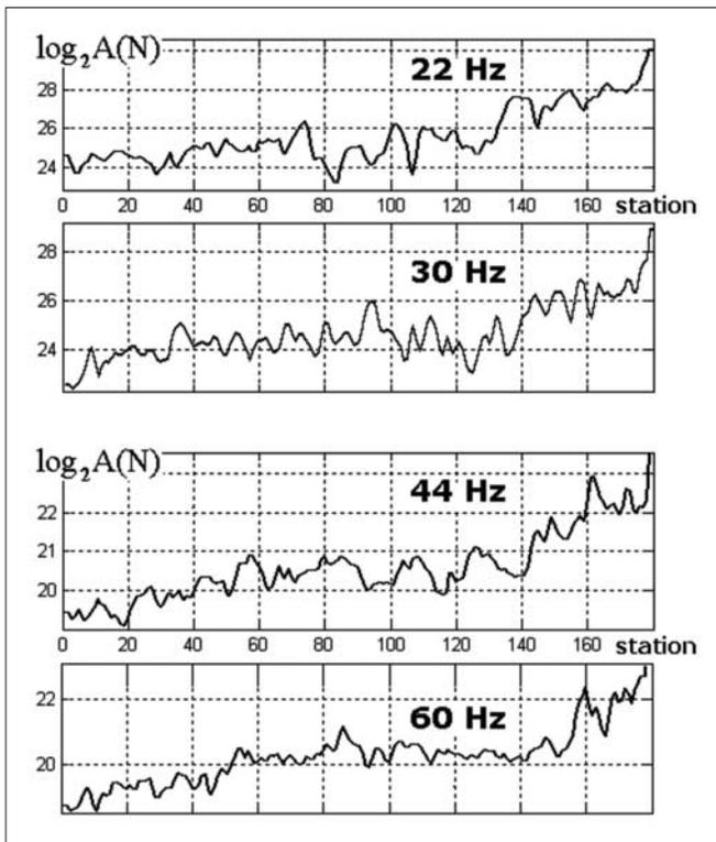
Figure 6. Amplitude variation of the base frequency and its harmonics. Both groups of vibrators are close to each other and at the end of the line.
