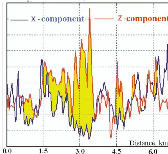
Fig. 1. The amplitudes values of the noise for X (blue graph) and Z (red graph) components along the test line.
