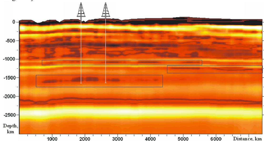
Fig. 5. Seismic emission depth section. The initial data were registered during an ordinary field-work.
