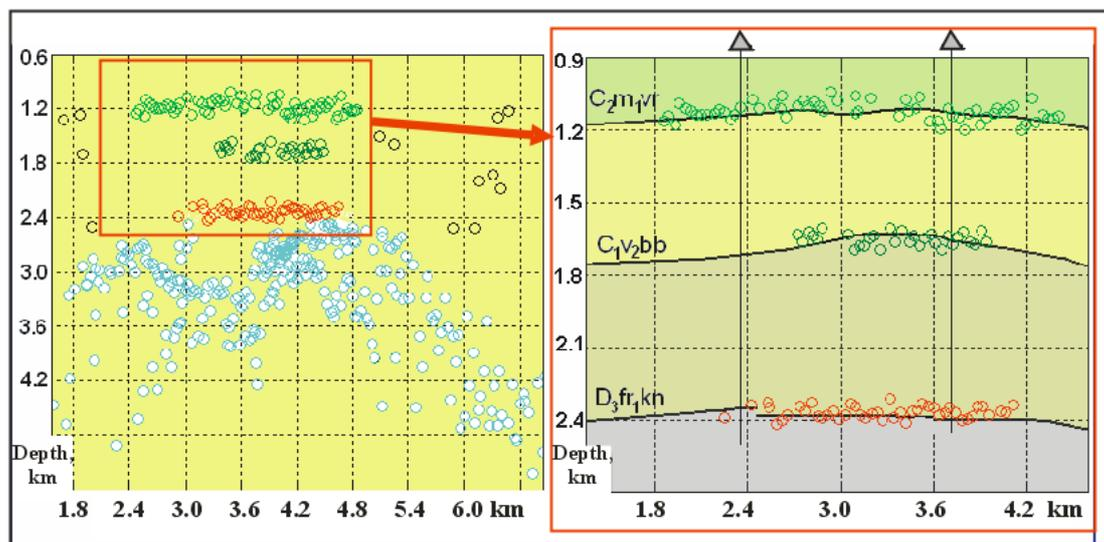
Fig. 3. The distribution of seismic emission sources after averaging their coordinates with specially defined zones.
