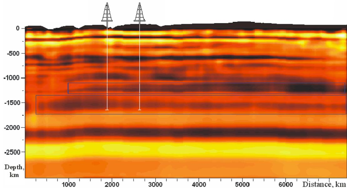
Fig. 4. Seismic emission depth section. The initial data were registered without special influence on the medium.
