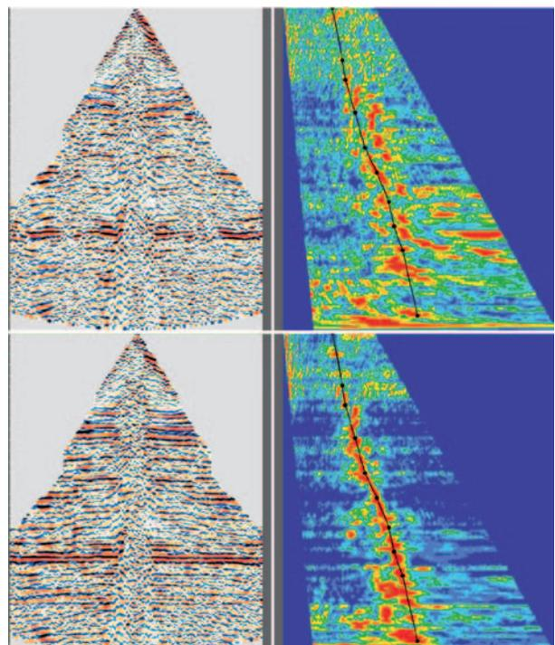
Figure 5 Velocity analysis before (top) and after (bottom) statics was correctly resolved.
