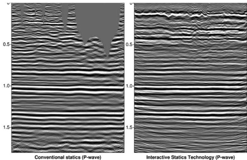
Figure 9 Conventional (left) and Interactive Statics Technology (right). Note improvements in the shallow section. Reservoir is around 1 s.
