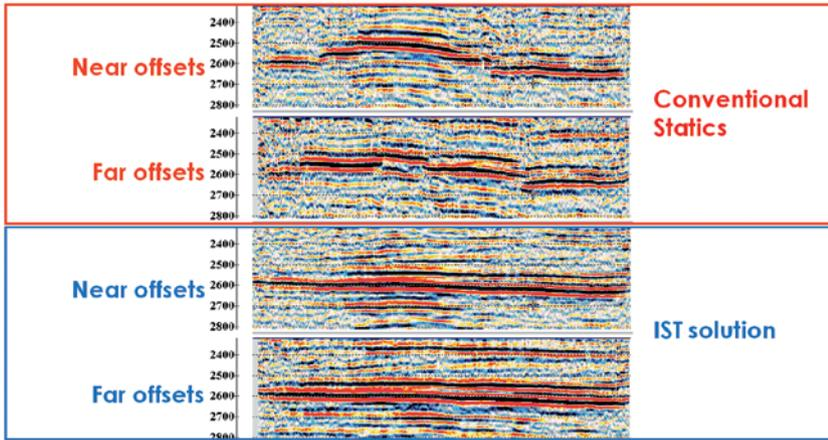
Figure 6 QC of the statics solution. Conventional velocity-based (top) shows a different geological structure on near and far offset stacks. Correct statics solution (bottom) obtained with IST shows the same structure on both offset ranges.
