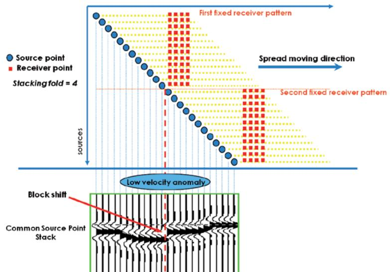
Figure 3 Spatially fixed pattern in 2D case. Note the block shift between the elements of the pattern due to near surface anomaly.
