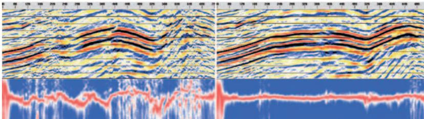
Figure 7 Horizon Velocity Analysis comparison between conventional (left) and Interactive Statics Technology (right).
