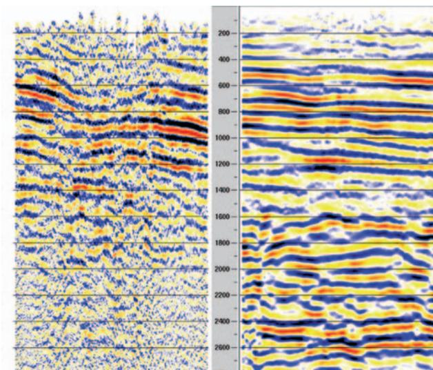
Figure 10 Initial (left) and final (right) stacks for mono type S-wave dataset.
