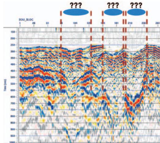
Figure 2 Common-offset section with all a priori statics applied. Undulations in first break energy and change in surface noise signature denote near-surface related anomalies.
