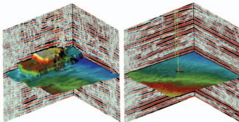
**Figure 1** Conventional statics solution (left) vs Interactive Statics Technology (right). IST was able to remove false structure due to large near-surface velocity anomaly.
