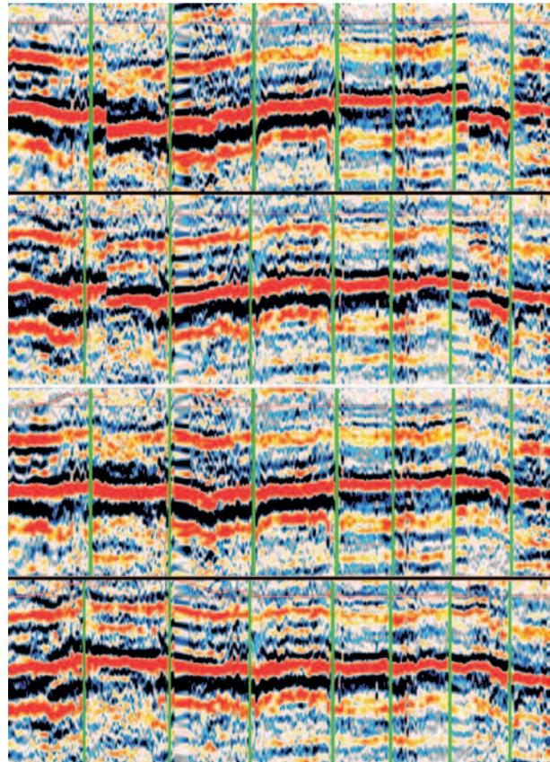
Figure 4 Spatially fixed patterns before (top) and after (bottom) statics corrections applied.
