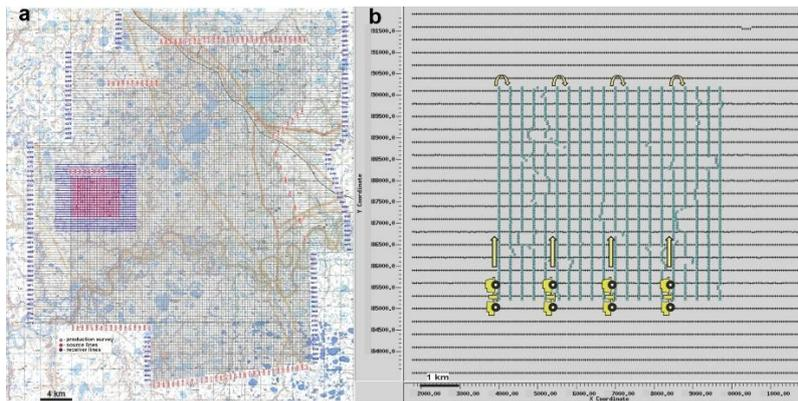
**Figure 2** (a) 3D production survey map (grey lines) and experimental survey layout (red and blue lines). (b) Vibrator groups moving (yellow figures and arrows) in the experimental Shuffle and ISS surveys.
